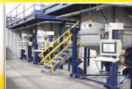
Silicon feedstock is melted and solidified inside a directional solidification furnace
